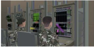
Figure 5. Two operators shown as avatars operating the BYG-1 Combat System. The operators were logged into the QwaqTeleplace Clients located in a different building as the combat system hardware. The system was effectively desktop sharing the combat system
